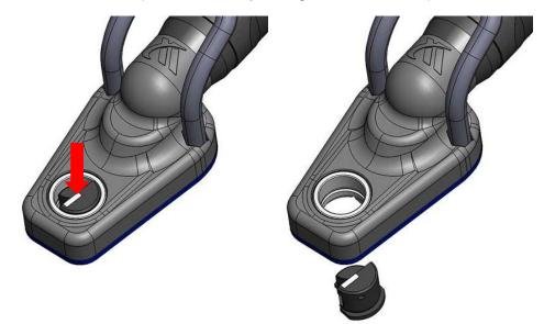
2. Remove the M3 torque screw from the Cutter / Holder and change the Cutter.
