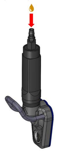
2. Run the dresser without pressure for 3~5 sec to lubricate.
