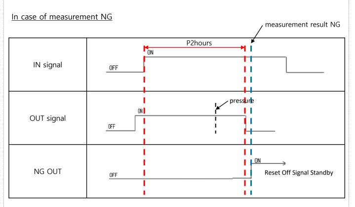
OUT signal is output to condition (combination) such as IN signal. e.g.) when IN1, IN2 input, above OUT signal is output from OUT1,OUT2.
