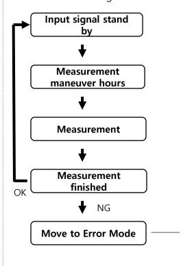
In case the P1 parameter is set to Auto Reset, When set hours, returns to measurement mode automatically.
