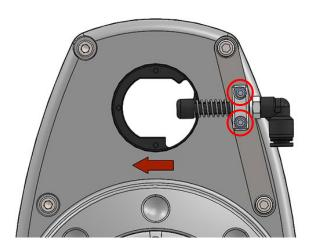
3. Attach the Solenoid Valve. (Use M5\*10 M5\*10 3-sems. Tightening torque 4.5N/m)
