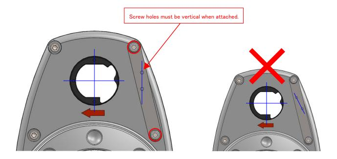
2. Attach Nozzle ASSY to the bracket. (Use M3\*14 Hex Socket Cap Screw, M3 Spring Washer. Tightening torque 1.0N/m)
