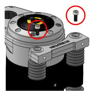
2. Draw out the lower shaft plate together with the shafts.
