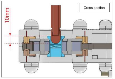
6. After inserting the cap tip into the center, and retreat it in the upward direction of the Z-direction.
