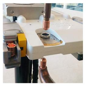
4. Adjust horizontal and vertical and move directly on the center of the teaching guide.
