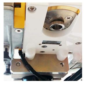
4. Finely adjust and insert the cap tip into the teaching guide about 10mm. If it is inserted correctly, horizontal and vertical are adjusted.
