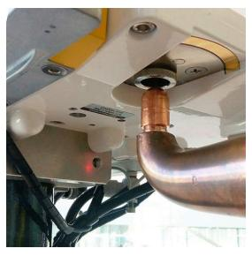
5. If it is inserted to the center, remove the teaching guide as above, Insert the cap tip again to parallel the surface of cap tip and remover.
