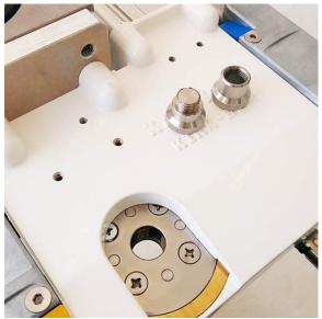
Insert the cap tip back into the center of the groove of remover, adjust the cap tip surface to parallel with the remover face
