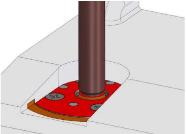
As shown in the picture on the right above, the center of the cap tip and the groove are adjusted as the cross -sectional view, if adjust aligning the cap tip surface with the remover face.
