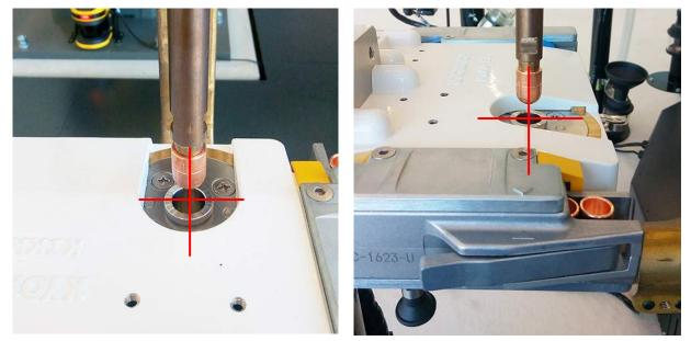
5. Finely adjust and insert the cap tip into the teaching guide about 10mm.
