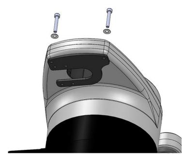
3. Mount a chip collector with 3-point sems bolt (M4-8L x 4pcs) on the adopter.
