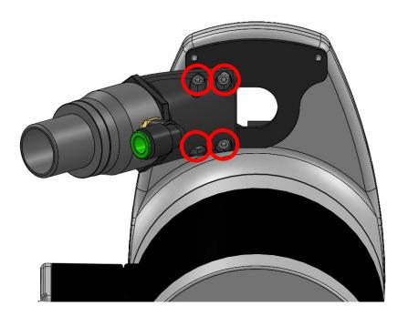
4. Attach hose and hose band to chip collector.
